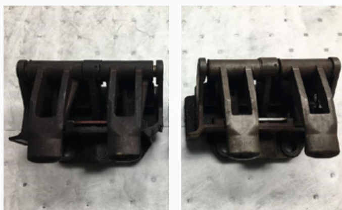
Fig. 5: Chain blocks before (left) and after (right) Ivey-sol surfactants were used to clean residue off the mechanisms.
