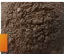
Hazardous free waste (Oil content \leq 2%)
