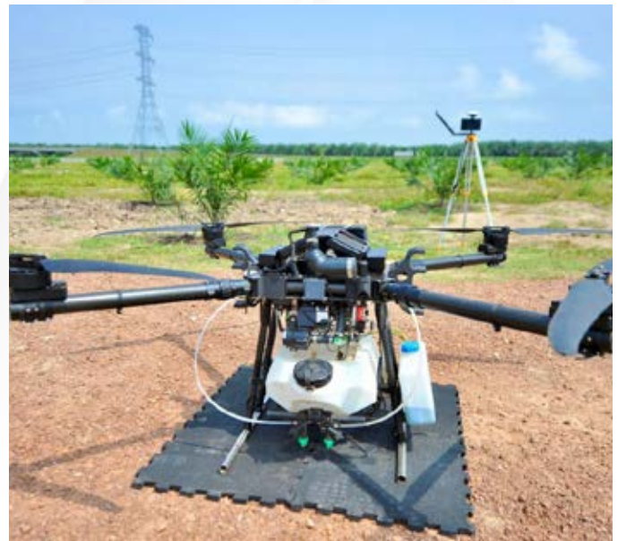
The Point-To-Point Drone Sprayer delivers extended hectareage precision spraying of pesticide based on crown tracking, using artificial intelligence
